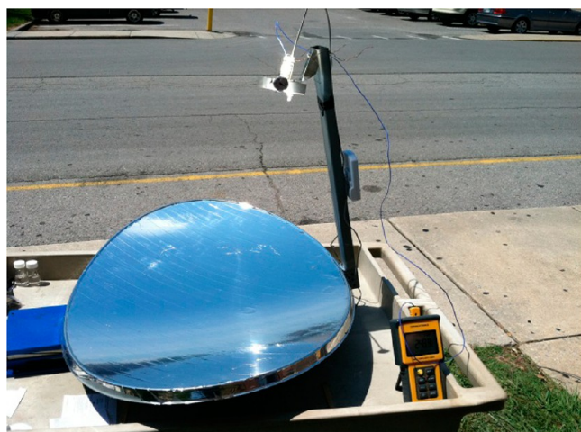
Figure 1. Repurposed satellite dish heat source.
